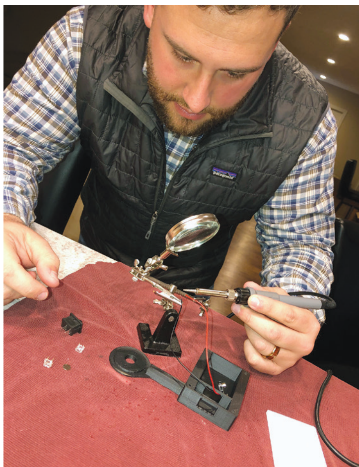
Drew Deathe solders electronic components for the 3D-printed scope, which can be attached to a mobile phone for use in assessing trachoma symptoms.
