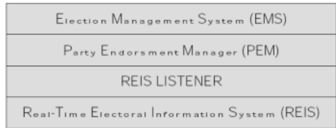
Figure 5: Tallying system modules (Source: CNE, “SAES_v3.2 101006.pdf,” 2006)
